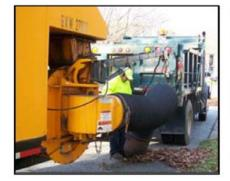
Visibility of the workers on foot is a critical component for a safe operation. In the picture on the left, the worker is between the leaf vacuum and the truck and out of the driver's sight.
